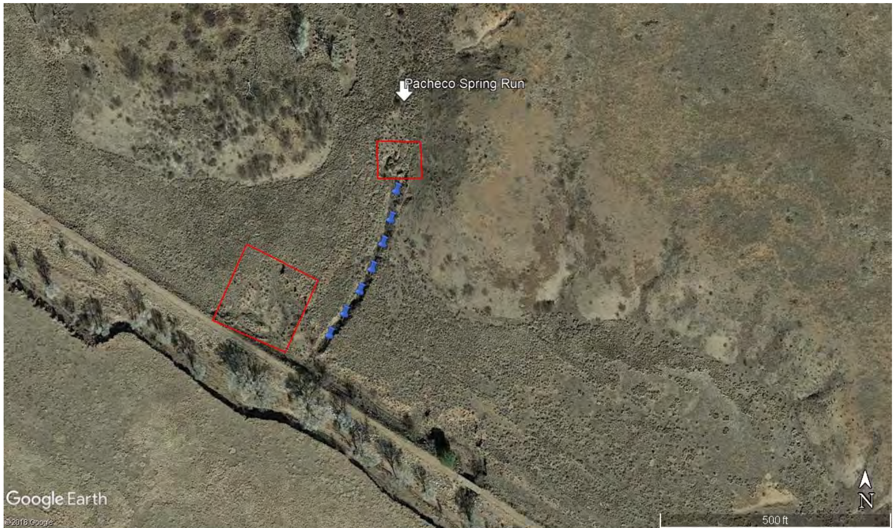
Pacheco Spring check dam locations and red polygons indicate previous work with media lunas and Zuni bowls
