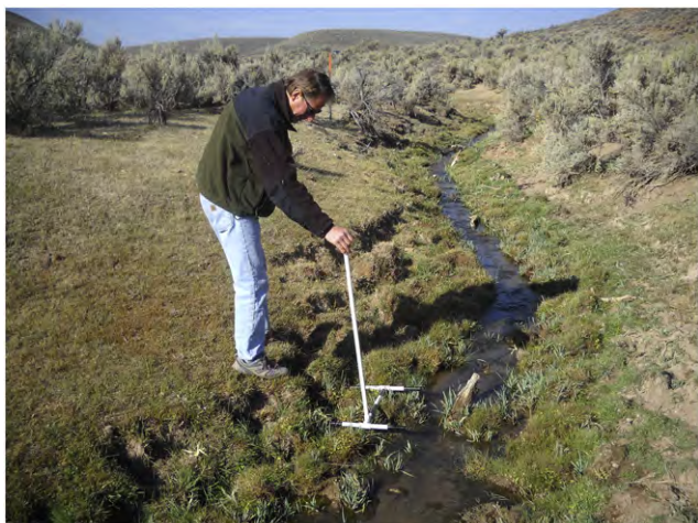
Figure 3. Measuring bank alteration and stubble height.
