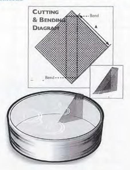
Figure 2: Expanded metal grating (with 1/2 inch mesh) is an effective wildlife escape structure. Use the cutting diagram with the length matching the depth of the rectangular trough. The ramp is bent and the top corners bend over rim of trough. Attach with screws and bolts.
