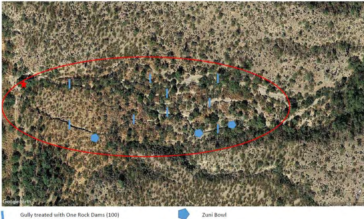
Figure C-6. Downstream Pantano Dam Site #3: Red oval is Area of Potential Effects, blue lines are channels for treatment with one rock dams, and blue pentagons are Zuni Bowls. The red star is the rock staging area on the second floodplain terrace. Rock delivery to structure sites will be by wheelbarrow.
