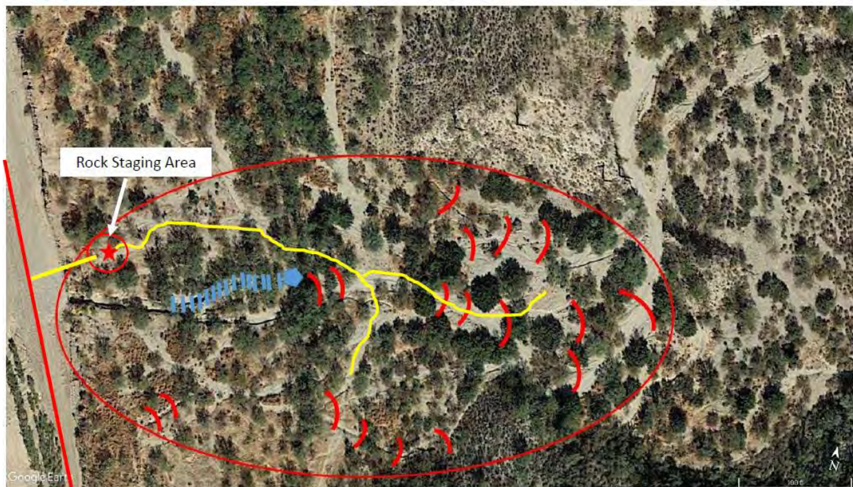
Figure C-5. Downstream Pantano Dam #2 site: Red oval is Area of Potential Effects, red arcs are Media Lunas, blue lines are one rock dams, and blue pentagon is a Zuni Bowl. The red star is the rock staging area on the first floodplain terrace
