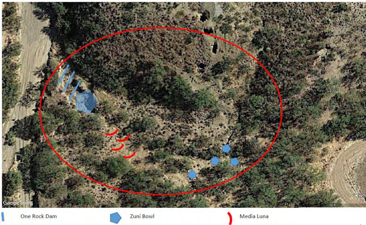
Figure C-12. Davidson stock tank erosion area design (note: orientation is rotated 90 degrees to the west)
