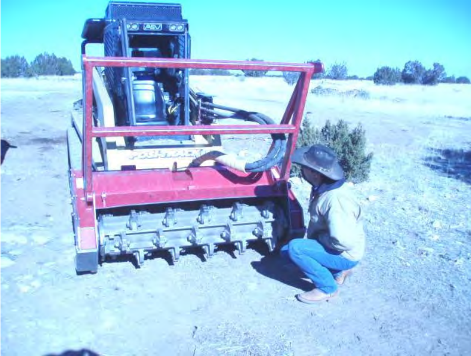
Figure 1. This is a photo of the roller chopper mounted to a skid steer loader large enough to handle the weight of the equipment.
