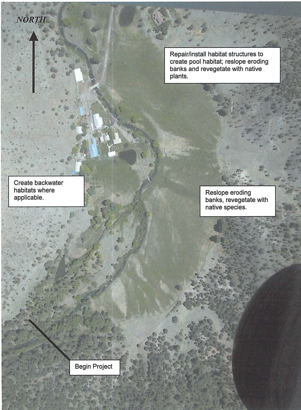
Figure 5. Project Reach 1. Stream channel is fairly well contained in this reach. Project activities are expected to include bank stabilization, repair/installation of rock structures for habitat, creation of overhanging bank habitat and revegetation where necessary.
