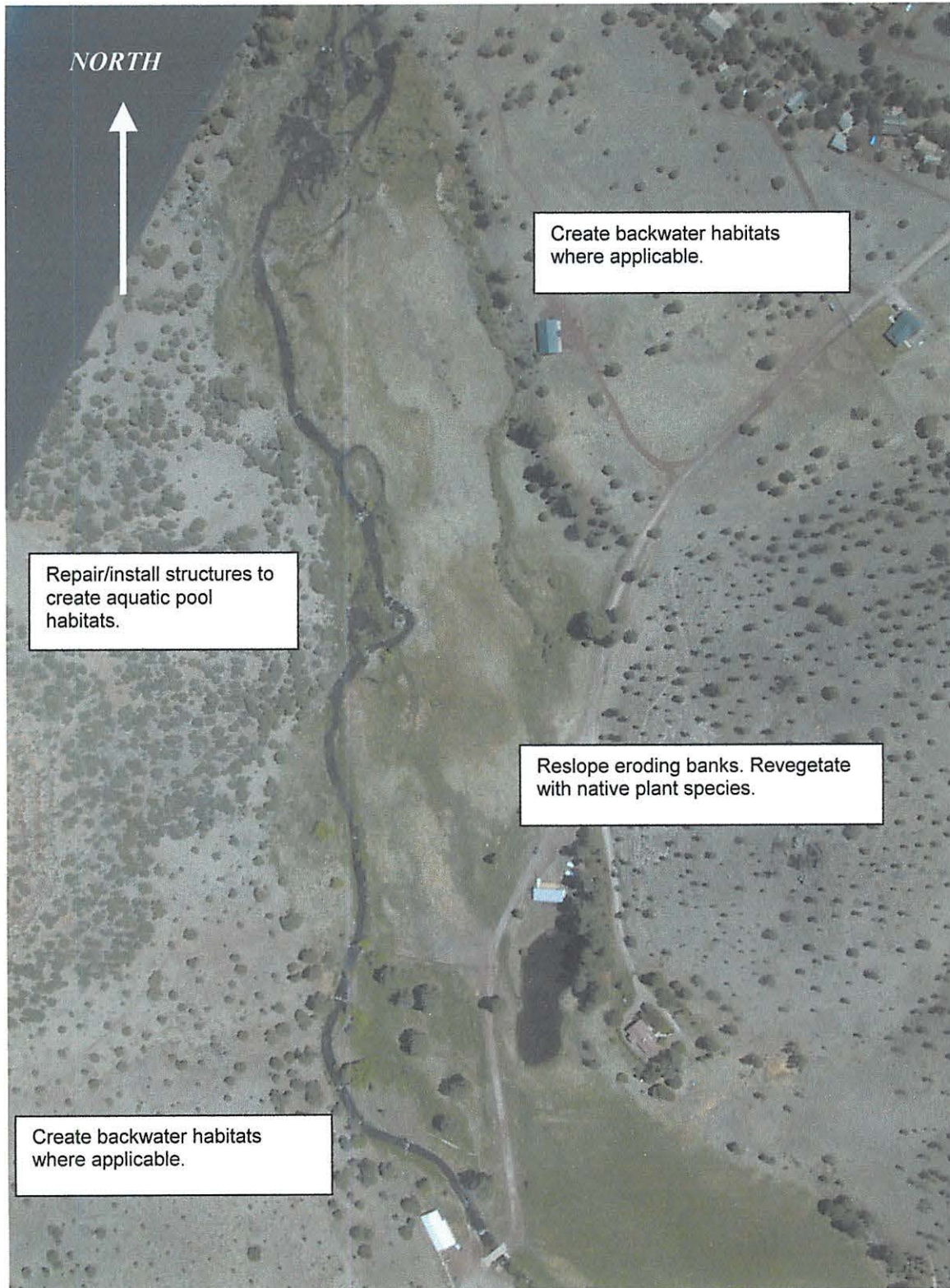
Figure 6. Project Reach 2. There is significant opportunity for creation of additional backwater and bank habitats in this reach. Eroding banks will be stabilized with bioengineering practices. Rock structures for pool habitats will be repaired/installed where needed. Backwater areas and overflow channels will be created and the reach revegetated as needed.
